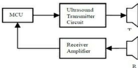
Fig.1. Block Diagram of Ultrasonic Sensor
